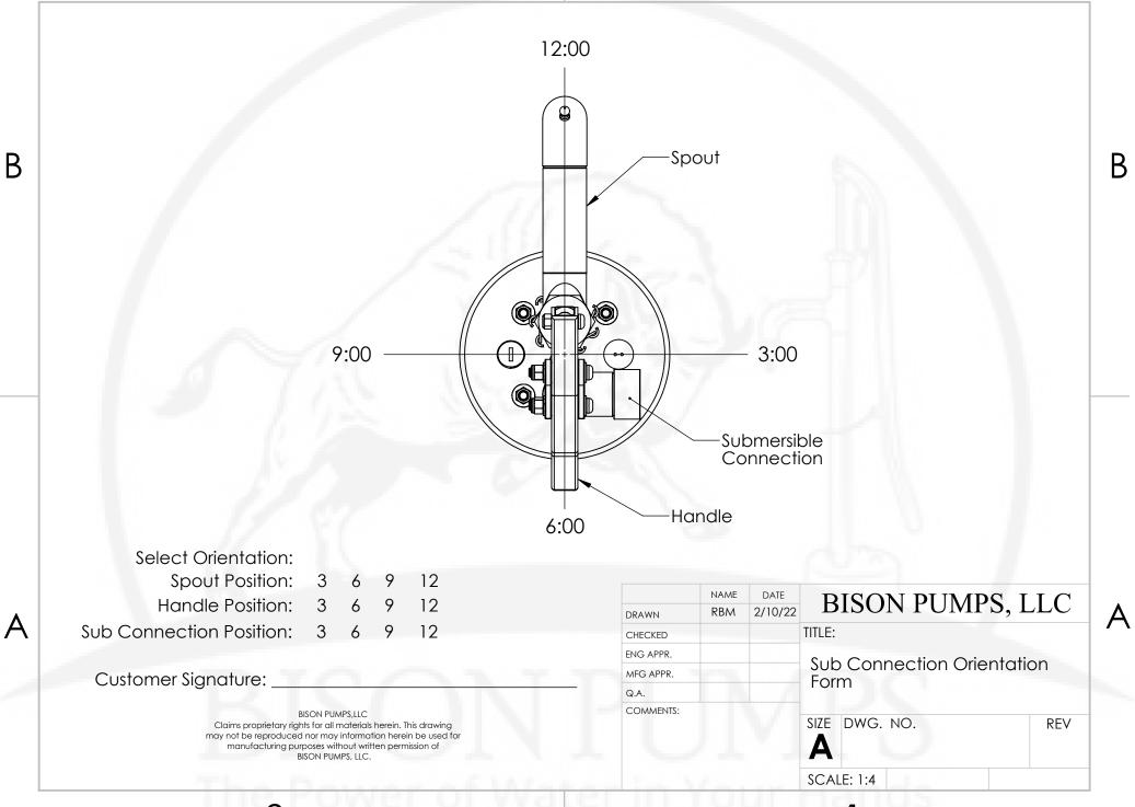
Submersible Connection Deep Well Pump Head Orientation Form
