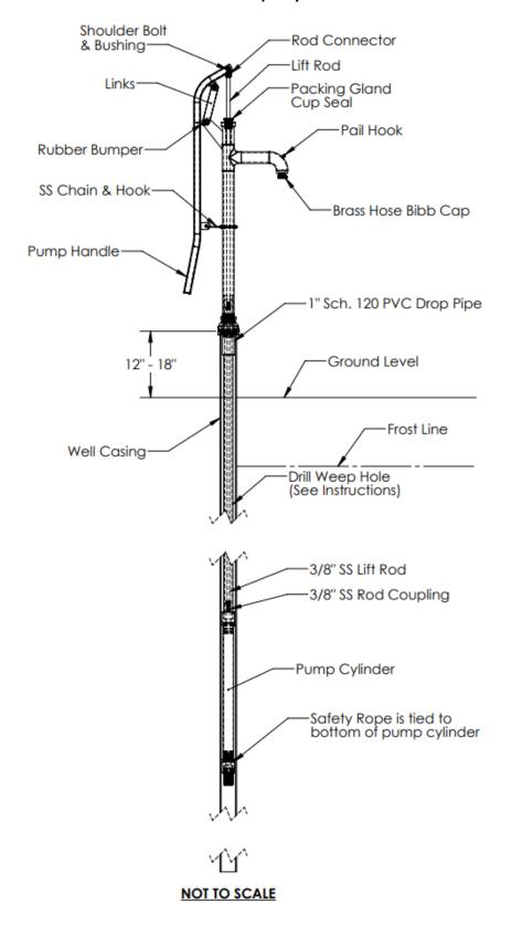
Detail B: Weep Hole Location Diagram
