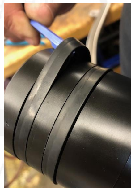
Photo 8.1 - Cup Seal Removal
