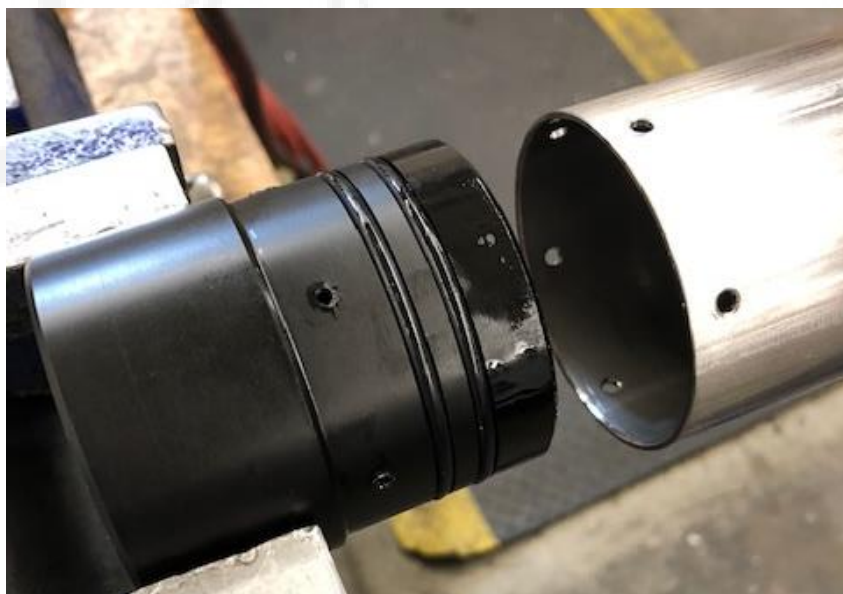
Photo 2 – Bottom End Cap Removal
