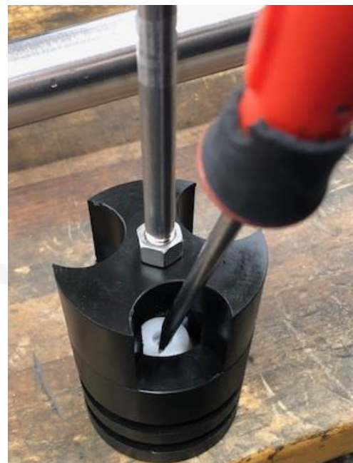
Photo 8.2 –Piston Check Valve Removal
