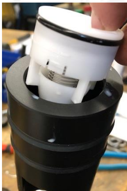
Photo 9 – Piston Check Valve Orientation
