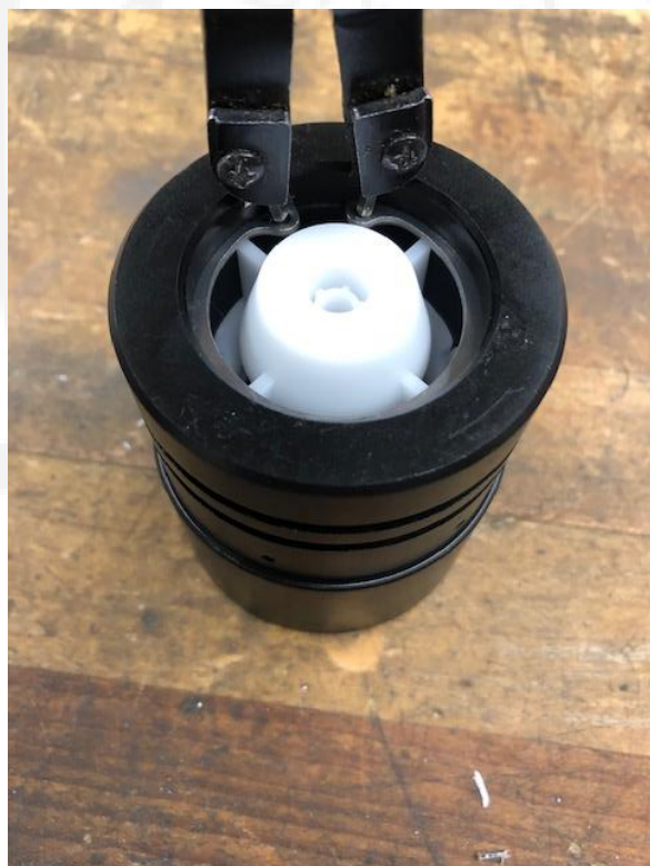
Photo 4 – Internal Snap Ring Removal
