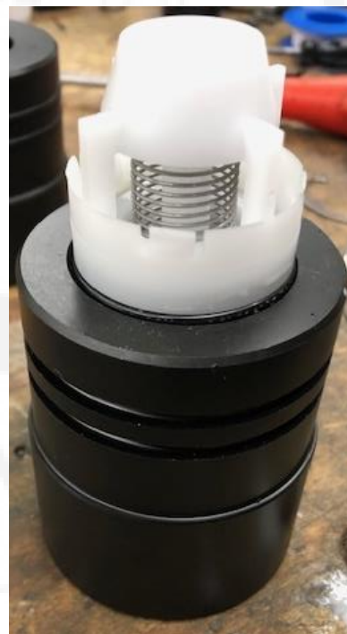
Photo 6 – Check Valve Orientation
