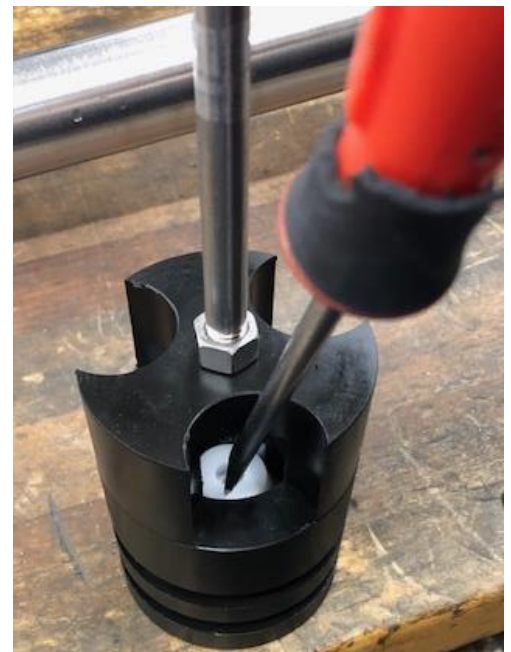
Photo 8.3 –Piston Check Valve Removal
