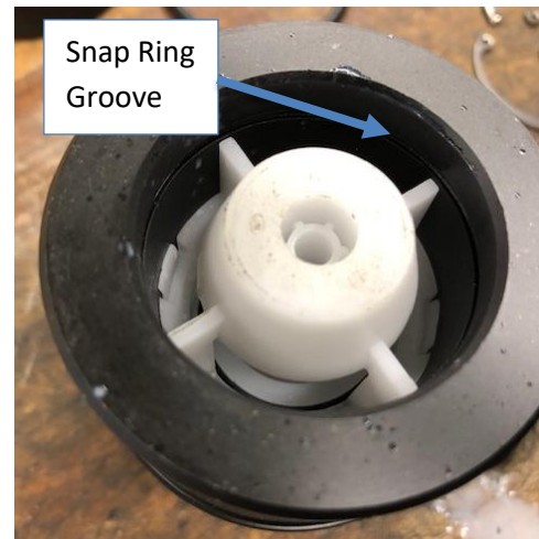
Photo 7 – Check Valve Placement
