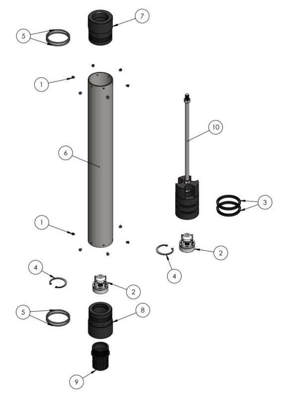
Detail G: Standard Cylinder Assembly Exploded View
