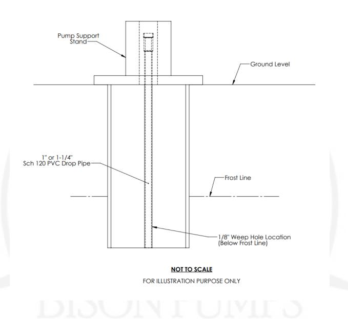
Note: Depending on Well Casing height, Pump Support Stand height, and the frost line depth it is possible for the weep hole location to be on the 2<sup>nd</sup> section of drop pipe instead of the 1<sup>st</sup> (the drop pipe connected to the pump head). Be sure to add the height to the top of the Pump Support Stand (from the ground) to the frost line depth to ensure the weep hole location is below the frost line.
